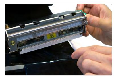
**Note:** Only the very front of the printhead needs to be cleaned with the cleaning pen. Take care not to damage the printhead especially if wearing jewellery. Never under any circumstance use a sharp object to remove excess waste from the printhead as this is likely to cause severe damage.
