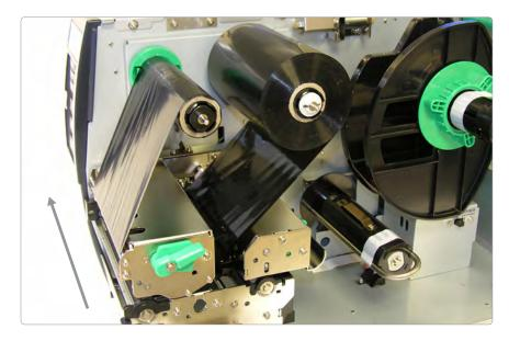
**Note:** If unsure about pulling the thermal ribbon across without tearing please remove the ribbon entirely and refit after cleaning. If the ribbon is torn it will no longer be usable and will have to be replaced.
